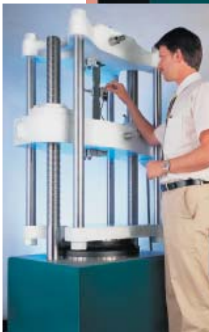
Fig. 6. Typical 60,000 lbf (300 kN) Super "L" with optional computer running Tinius Olsen's Test Navigator software.
