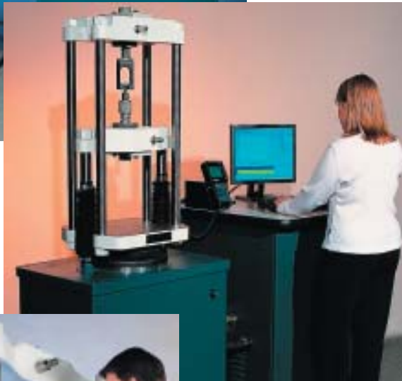
Fig. 6. Typical 60,000 lbf (300 kN) Super "L" with optional computer running Tinius Olsen's Test Navigator software.
