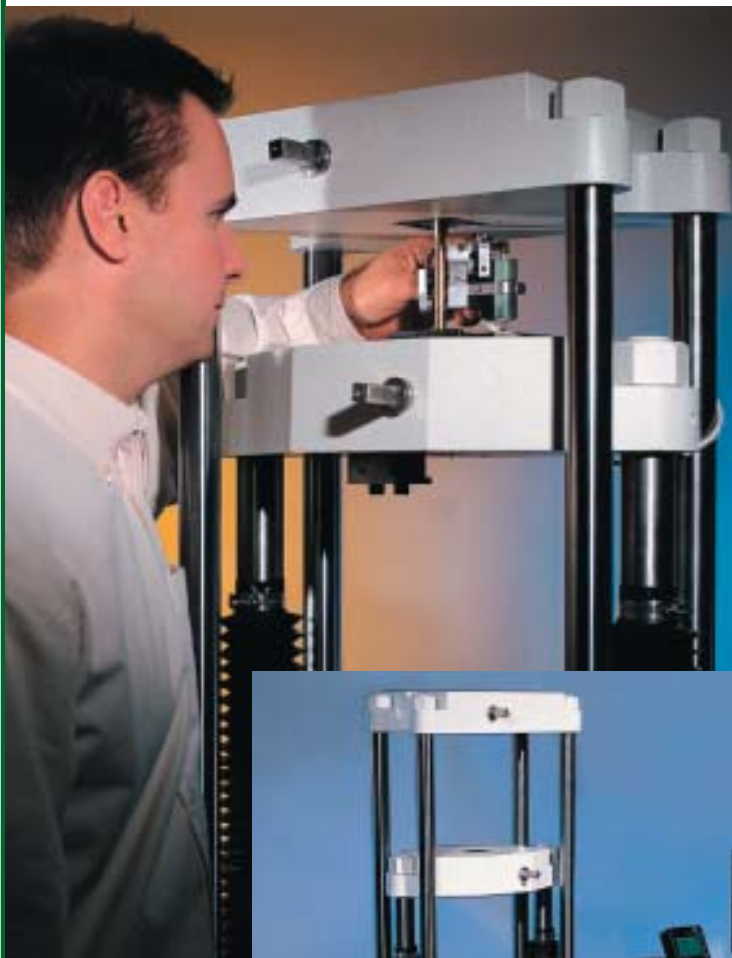
Fig. 1. Typical 60,000 lbf (300 kN) Super "L".
